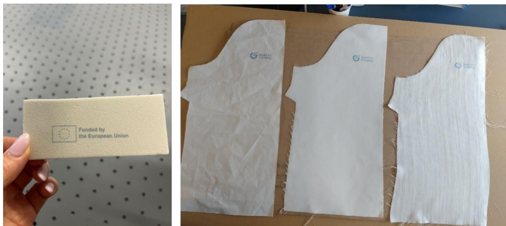
Figure 5 Foam (left) and PHA-coated textile (right) samples printed using the bio-based ink formulation.
