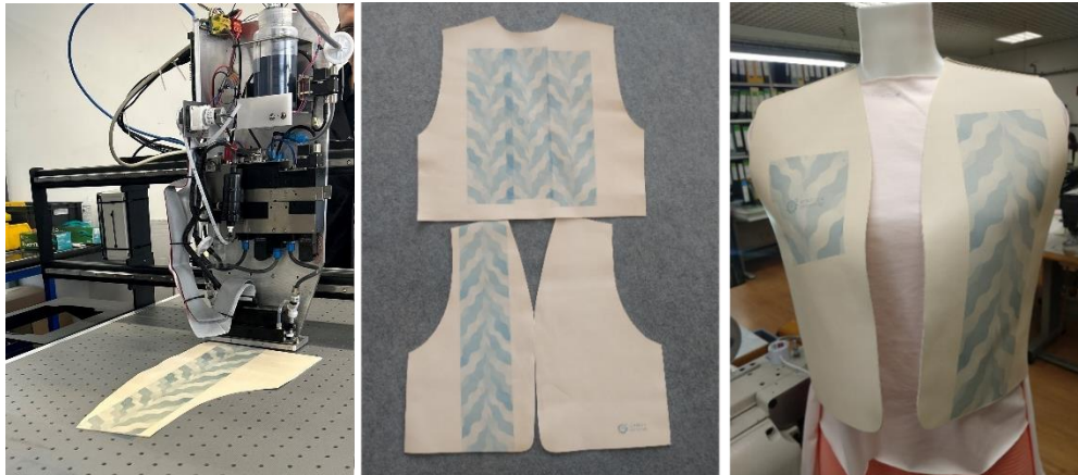
Figure 3 Printed leather pieces prior to assembly into a sleeveless vest.
