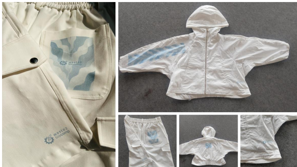
Figure 2 Demonstrator garments, including a jacket and a pair of shorts, printed using the 2D inkjet system developed within the project.
