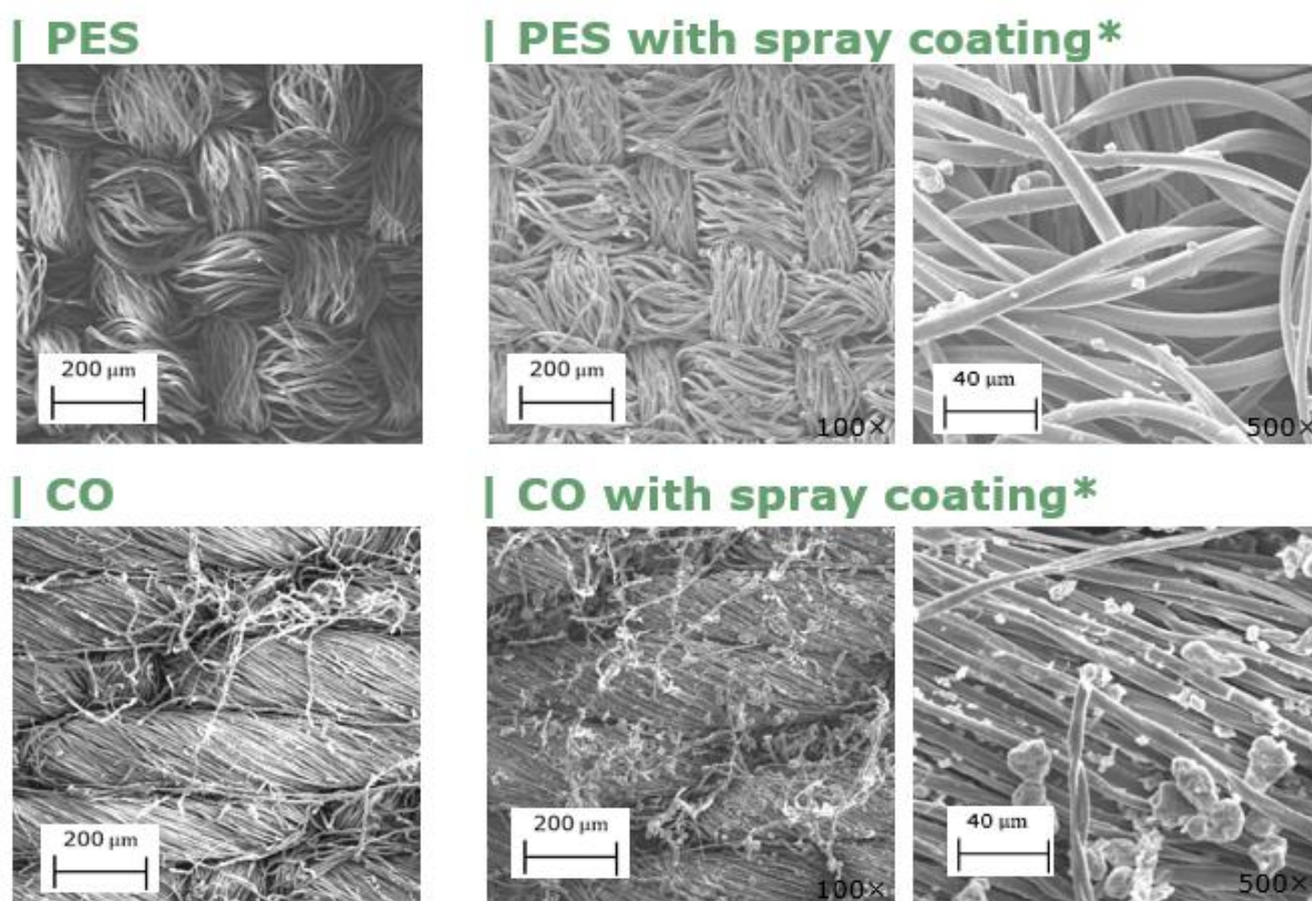
Figure 2 SEM micrographs of PHA-coated polyester and cotton control fabrics. The left images represent the control and those at right presented the coated substrates.
