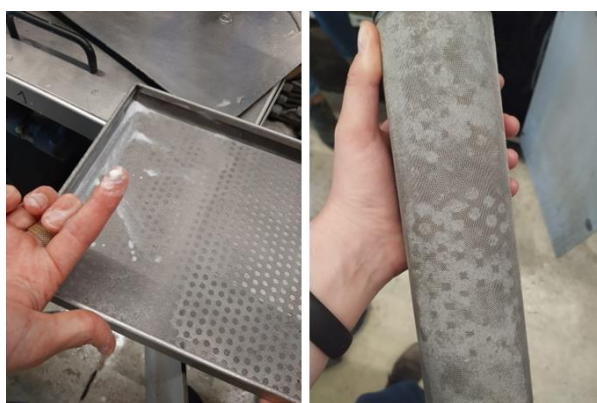
Figure 8 Clogging issues encountered during the spray coating process.
