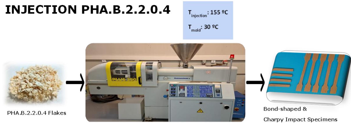
Figure 10 Injection process and parameters used for PHA.B.2.2.0.4 flakes.
