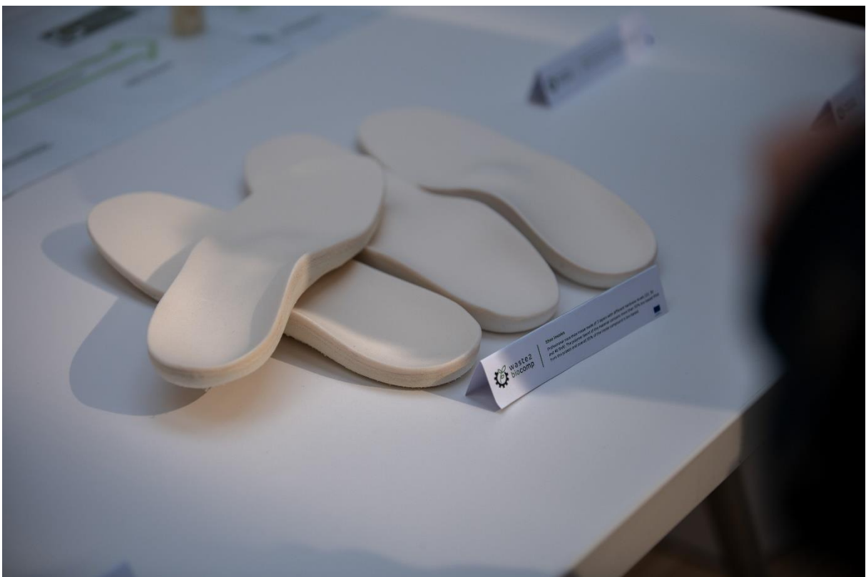
Figure 1 Three-layered medical shoe insoles developed with the PHA-based foams developed in W2BC .
