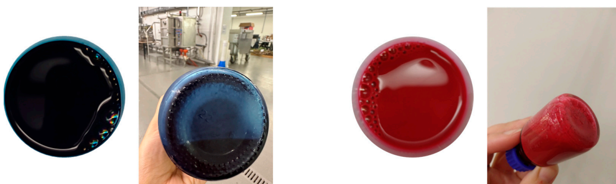
Figure 1. Inks made with 1.0% indigo pigment (left) and 0.5% quinacridone pigment (right) in powder form and their respective deposits.
